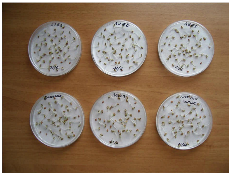
Fig. 8: Picture of the cress seeds germination test
